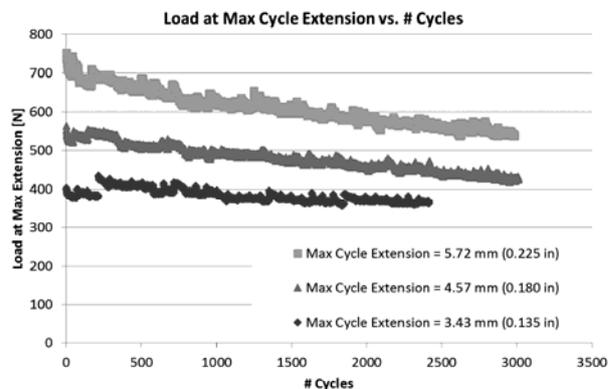
Fig. 3 Variation of the peak load with number of cycles during the cyclic three-point bend test. Three maximum bending displacements are prescribed: 5.72mm, 4.57mm and 3.43mm
