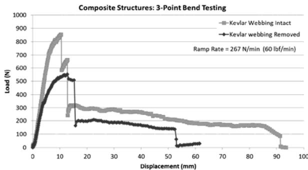
Fig. 2 Load-displacement response of the specimens with and without the external Kevlar weaves, during monotonic three-point bending
