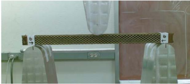
Fig. 1 (a) Schematic of the composite beam specimen. (b) An actual specimen and the three-point bending experimental setup
